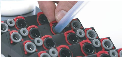
**Insert-and-Seal feature combined with modular design provides quick and easy color change**
