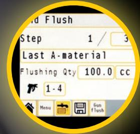
Function "Last A material" prevents sticking of the valve seat and thus avoids a standstill.
