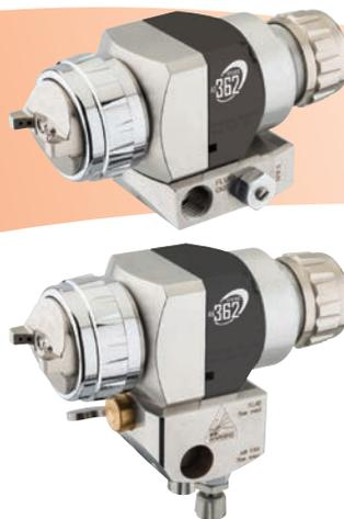
Built to the same superior specification as the AG-361 automatic guns but with the addition of a quick detachable Manifold base. This allows the gun to be quickly and easily removed for maintenance, cleaning or change-over without disturbing the positional settings. On re-attaching the fluid and air can be turned back on and the gun is instantly in the right location ready for operation.
