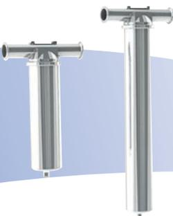
The Binks range of cartridge filters remove dirt and paint clots from paint systems using a choice of disposable or cleanable filters elements. They allow the rapid replacement of the elements with their "fixed in place" clamp design. The housing also provides an integral pressure gauge port to allow for the measurement of differential fluid pressure.
