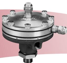
The Ransburg DR-1 Fluid Regulator provides constant fluid regulation for automatic coating application systems. It features two selectable fluid pressure ranges, low and high. The low flow range output provides precise fluid delivery control and the high flow range output accommodates higher fluid deliveries. The combination provides excellent paint film uniformity with minimal colour change time.
