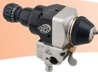
A modified manifold mounted gun designed for the precision application of coatings onto cosmetics packaging and glassware. The gun utilises 'Petite' precision air caps and fluid nozzles specifically designed for this style of application. For extra-fine fluid control the gun is fitted with a Micrometer vernier needle control knob assembly that allows ultra-fine precision fluid setting.
